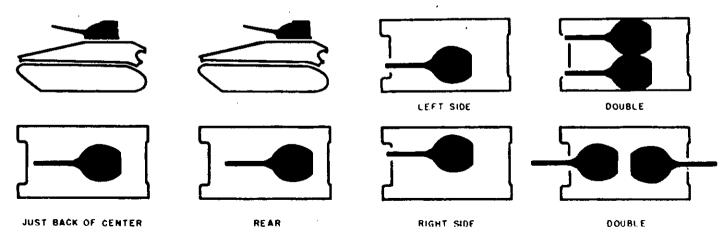
FIGURE 1. Position of turret on hull.
