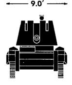
Armament: One 40-mm AA gun. Traction: Full track; five large evenly spaced bogie wheels; rear driving
