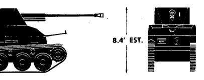
INTEREST DATA: This is an ex-Czech chassis which the Germans have used effectively as a self-propelled gun mount. Many vehicles mount captured Russian 76.2-mm guns, others German 75-mm guns. One type has a low hull superstructure and very large gun shield resembling a pyramidal turret. In all models the main armament mounts a muzzle brake and projects well beyond the front of the hull. The chassis is rather light for so large a gun.
