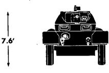
INTEREST DATA: This car is built in the United States for the British. It has been given the name "Staghound." The vehicle is classed as a medium armored car. It is equipped with a smoke projector on the right side of the turret roof.
