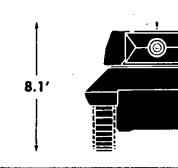
INTEREST DATA: This vehicle mounts a 3-inch gun in a turret on a modified M3 medium tank chassis. It has been the standard tank destroyer weapon, but is being replaced by the T70. It performed well in North Africa, where it was of great assistance in stopping German tank attacks.
