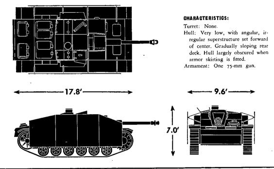
Traction: Full track. Six evenly spaced bogie wheels sprung independently. Large driving sprocket in front, large idler in rear.
