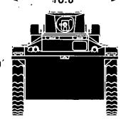
vertical sides covered by pontons; front and rear curve, "rocker" fashion, abruptly down to bogie assemblies.
