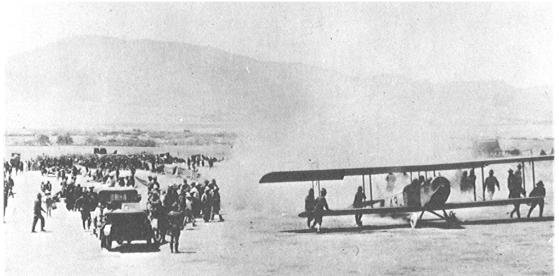
Aircraft #43, landing in Mexico during the Punitive Expedition, was one of the JN-2's converted to JN-3 by expanding the top wingspan and otherwise stabilizing the aircraft.
